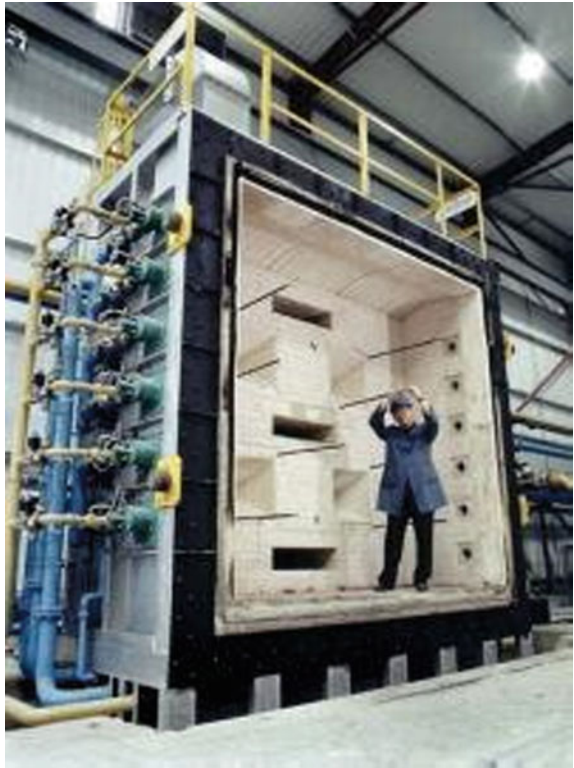
Fig. 6.24 Fire test furnace with gas burners at the side. The tested building structure is inserted air-tight in the front opening. The temperature in the furnace is increased by burners according to the “ISO 834” temperature–time curve [22]
