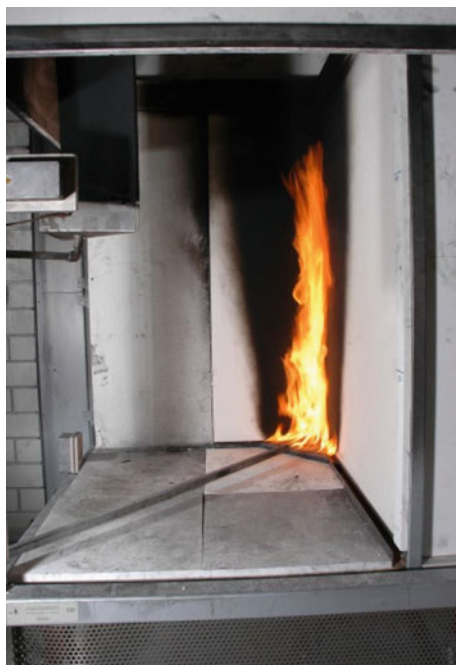
Fig. 6.13 In the test according to SBI (Single Burning Item) method, the corner of the apparatus is lined with specimens of tested material, which are then heated with a gas burner. The building material's reaction-to-fire class is determined by analysing the heat release and smoke soot, as well as by observing the flaming debris falling from its surface [17–19]
