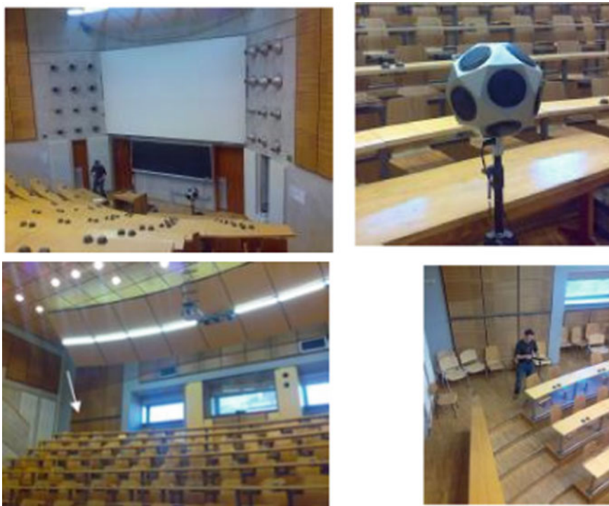
Fig. 5.41 Plečnik's lecture room at the Faculty of Architecture, University of Ljubljana. An isotropic source of pink noise that emits sound evenly in all directions was used as the sound source (top, right). Sound-pressure level was measured at two places, in the corner of the first and the last row (right)
