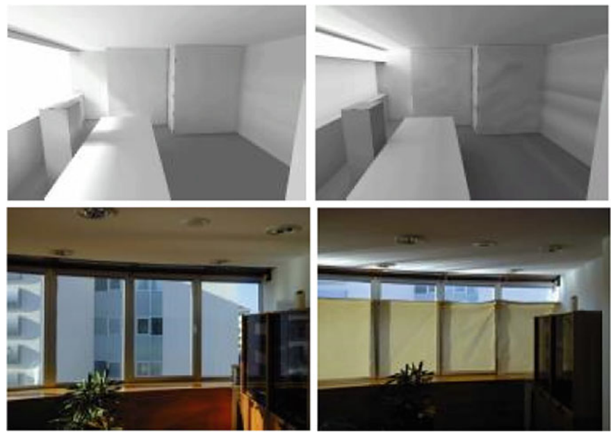
Fig. 4.65 Light shelves redirect the light deeper into the room. In the presented case the uniformity of the illuminance ( E_{min}/E_{av} ) improves from 1:6 to 1:3.5 [22]
