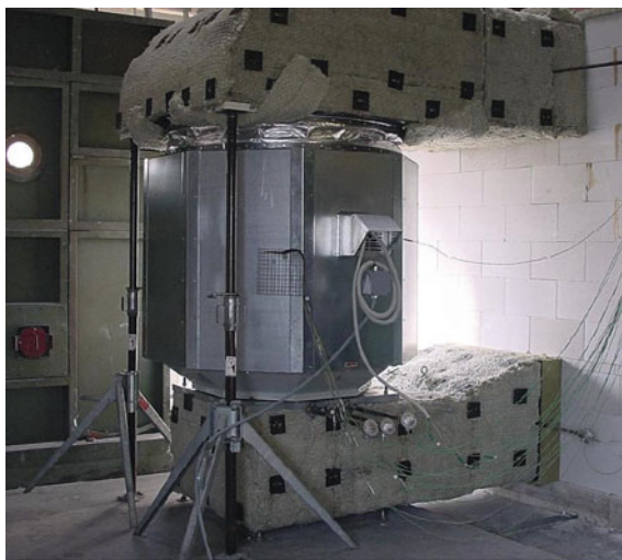
Fig. 6.30 As is the case with building structures, the fire resistance of the fans used for smoke extraction has to be tested too. Fire-resistant fans are divided into classes: a F200 class fan operates for at least 120 min with a smoke temperature up to 200 °C, while a F842 high-temperature resistant fan must operate for at least 30 min with the smoke temperature up to 842 °C [25]
