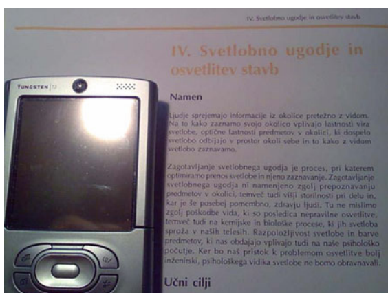
Fig. 4.67 High contrast caused by bright patch on the screen makes it difficult to read the text in the book
