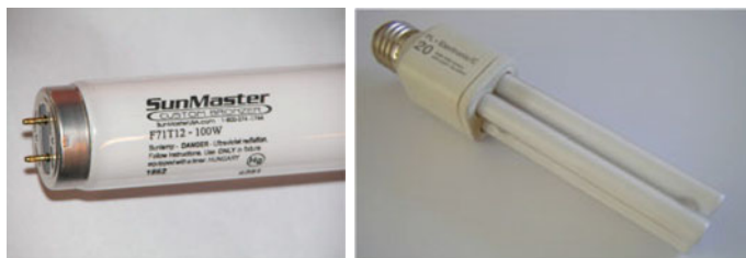
Fig. 4.46 Fluorescent lamps contain mercury vapour, which requires special disposal and recycling; the presence of mercury must be marked on the lamp (left); a compact fluorescent lamp is fitted with a silent electronic ballast and the Edison screw fitting to facilitate the replacement of old incandescent light bulbs (right)
