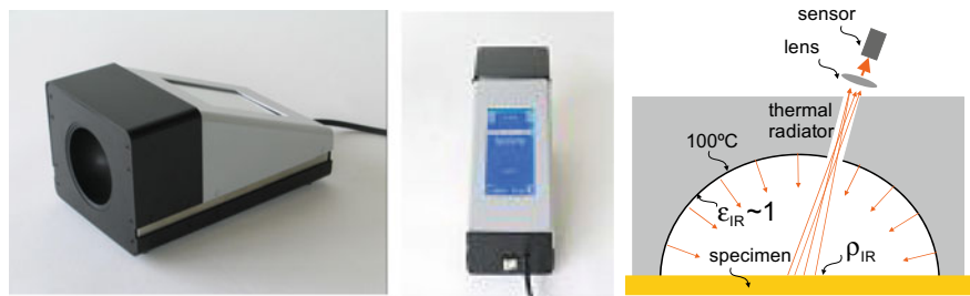
Fig. 1.29 Simple apparatus with a hemispherical heater, used for measuring the integral emissivity of thermal radiation \epsilon_{IR} ( 2.5 \mu\text{m} < \lambda < 40 \mu\text{m} ) (left, middle) and the measuring principle (right)
