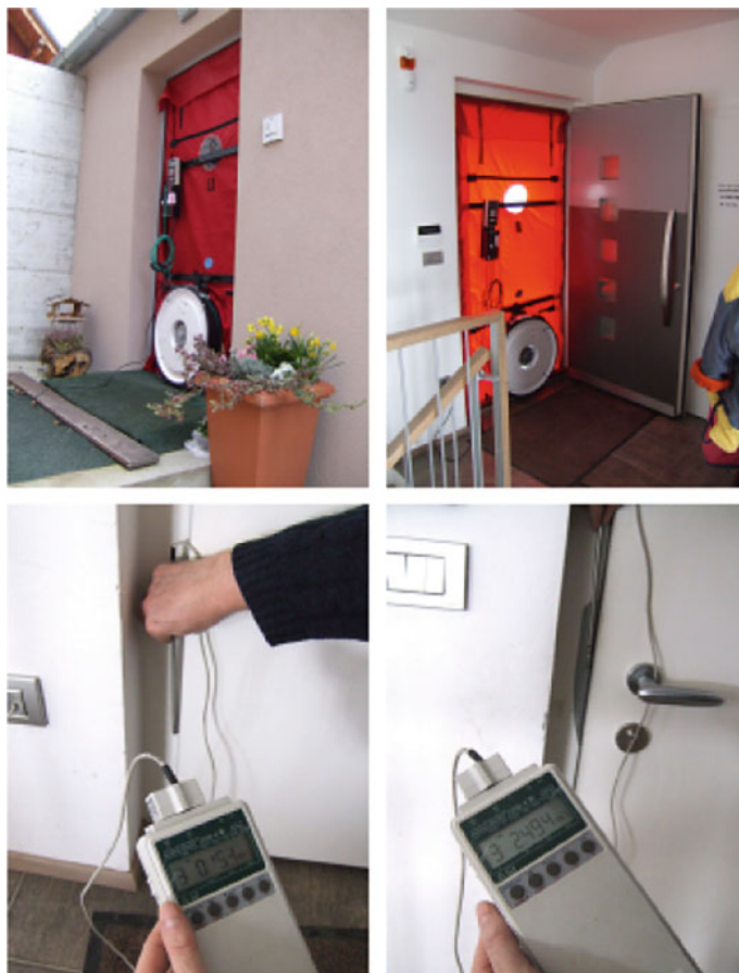
Fig. 2.20 The blower and the door panel system are sealed into the doorway, overpressure and underpressure airtightness test is done by rotation of the device (above); the untight point are detected by smoke generator or by velocity sensor; at pressure difference of 50 Pa, the air velocity on the site of the leakage can reach several m/s (below)
